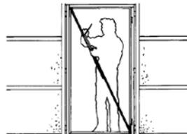
6. Mark the points of fixation on to the wall. Remove the frame, drill holes for the dowels and install the dowels into these. In case of timber structures the marking and drilling steps are skipped.
