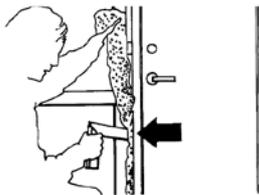
When finishing the protect frames with painting tape and door leaf with packing film. Fill the gap under the threshold with wooden blocks or wedges to prevent its deflection from later exploitation. Do not use installation foam or other elastic materials under the unsupported threshold.
