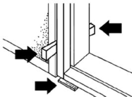
5. By using the spirit level, check if the frame is straight and level in vertical plane and the corners right-angled. Adjust with wedges, if needed. As shown in the figure, it can be checked whether the frames are installed in a right angle.
