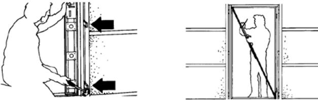
6. Mark the points of fixation on to the wall. Remove the frame, drill holes for the dowels and install the dowels into these. In case of timber structures the marking and drilling steps are skipped.
