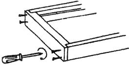
4. Lift the frame to the opening and fix with wedges. Install the wedges near the screws, see drawing. If ready-made floor level or on there is a need for more than 10 mm between the door leaf and floor level, you must also mount wedges under to the ends of threshold and/or vertical frame.
