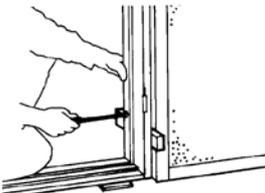
9. Install the leaf via the hinges on the frame and check with the leaf and spirit level that the frame opposite is in place. Adjust screws and/or wedges, if needed. If the door opens and closes without problems, also fix the opposite frame firmly onto the wall.
