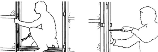
10. Check that the movement gap between the leaf and frames is equal in perimeter. Adjust screws and/or wedges, if needed.
